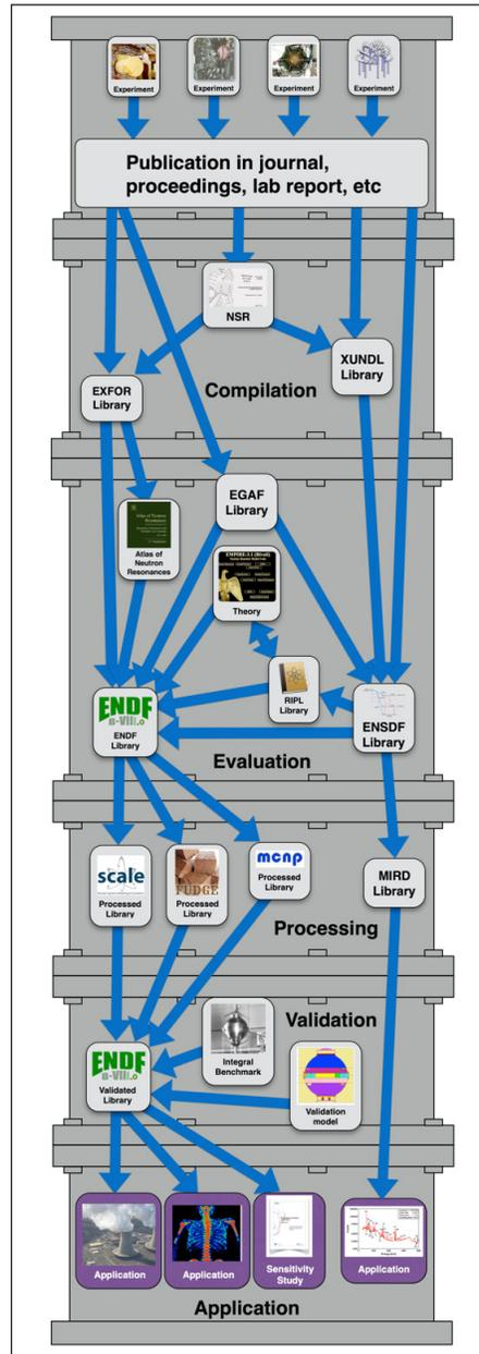
**Figure 1. The nuclear data pipeline. This is the process by which a nuclear reaction or structure measurements are converted into data tables for use in applications.**
