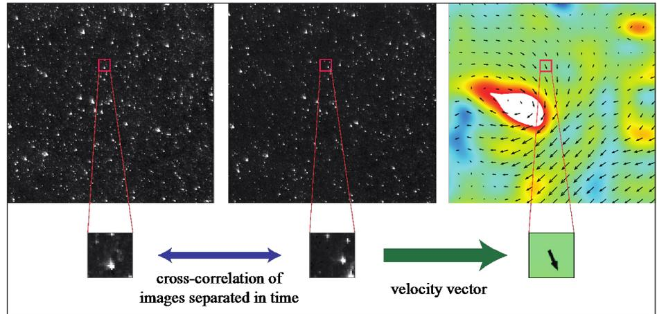
**Figure 1.** Images obtained with optical PIV, taken a short time apart (left, middle), can be subdivided into smaller images and cross-correlated to yield a velocity vector field from which quantities such as vorticity can be calculated (right).
