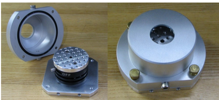
Figure 1. Gasket mounting plate and assembled canister.
